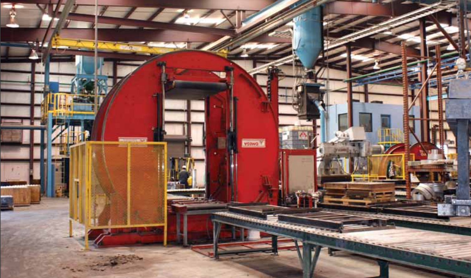
EBAA produces only its largest retention rings, as well as the flexible earthquake joint, on this manual nobake line.
