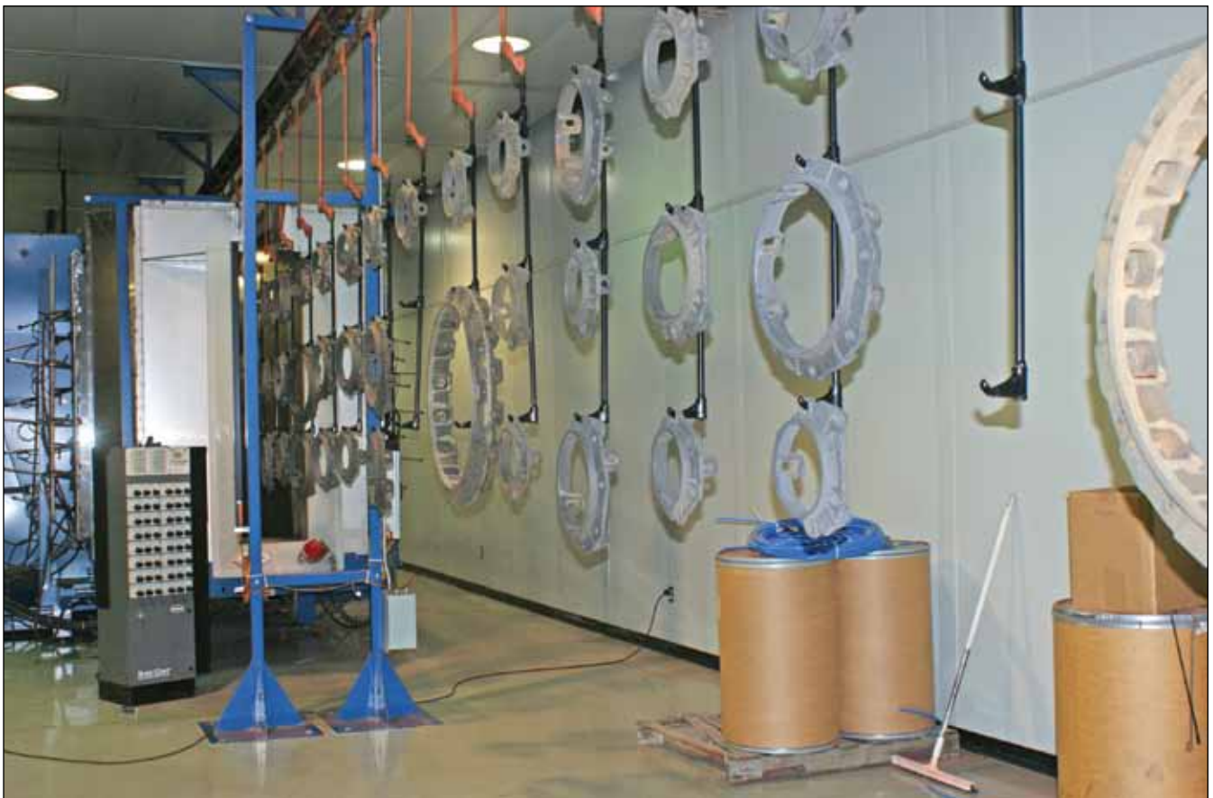
In addition to the new nobake plant and automatic grinding cells, EBAA installed this automated powder painting line to improve working conditions, increase productivity and produce a nicer finish.
